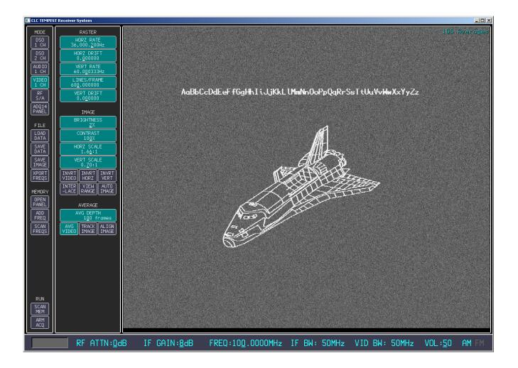
The application window can resized to fit the size of display used. The spectrum analyzer, oscilloscope and image windows are resized to the application window size. This allows better resolution when a high resolution computer display is used. The video image can also be dragged and zoomed using the mouse to provide better detail of any part of the video image.
