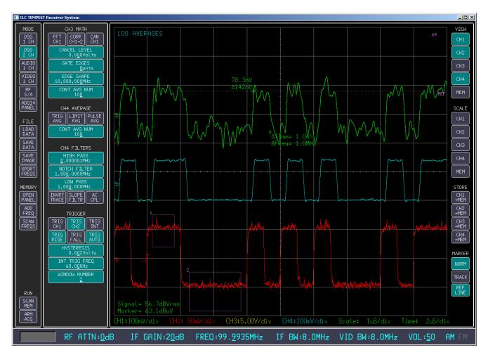
When running live, the traces provide persistence for visual correlation. The demodulated green trace also displays the range of values for signals represented by one pixel on the display. This allows the detection of fast signals in slow time bases that can be missed by conventional digital oscilloscopes.
