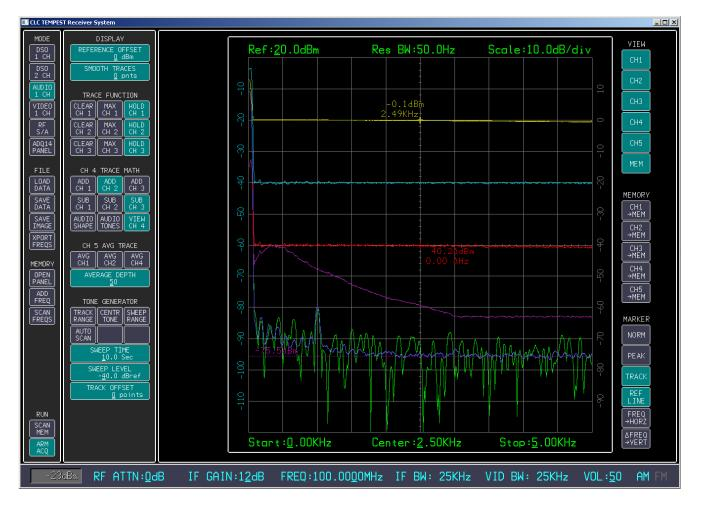
Graphical controls are used for the oscilloscope and the spectrum analyzers. The traces and markers can be dragged and expanded using the mouse. Markers are can also be used to automatically track the selected signal or find the peak and minimum value of the traces.
